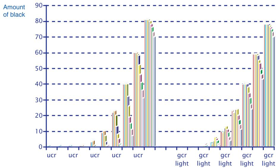
The comparison between UCR and GCR light in the red area of test form - Adobe Photoshop. From figure 6.
