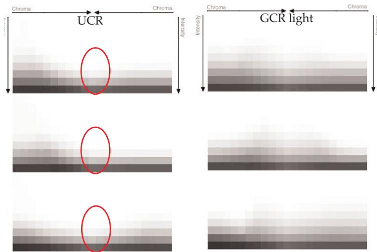
Figure 6: The difference between UCR (total ink limit 320, black limit 100) and GCR light (total ink limit 320, black limit 100)<sup>11</sup>. The red circles show the area where UCR should work according to the manual. For more information about values see appendix 1, 2 and 3.
