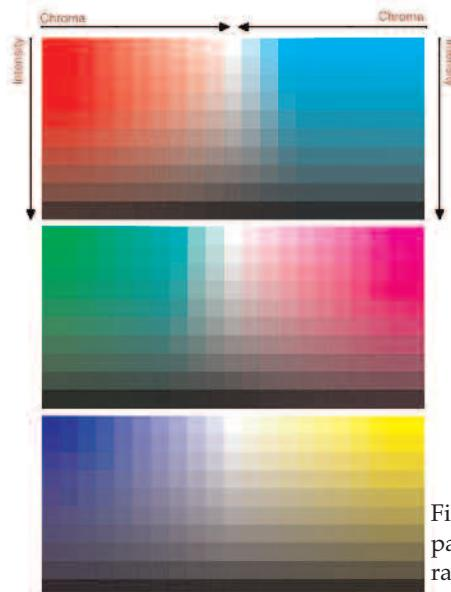
Figure 5: The test form. Moving from one patch to the next represents a change in saturation and lightness by ten percent.
